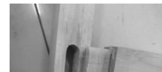
Figure 7. Specimen failure mode when \beta=0.2 mm
