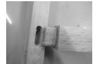
Figure 7. Specimen failure mode when \beta=0.2 mm
