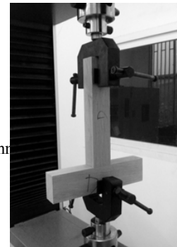
Schematic diagram of specimen clamping.
